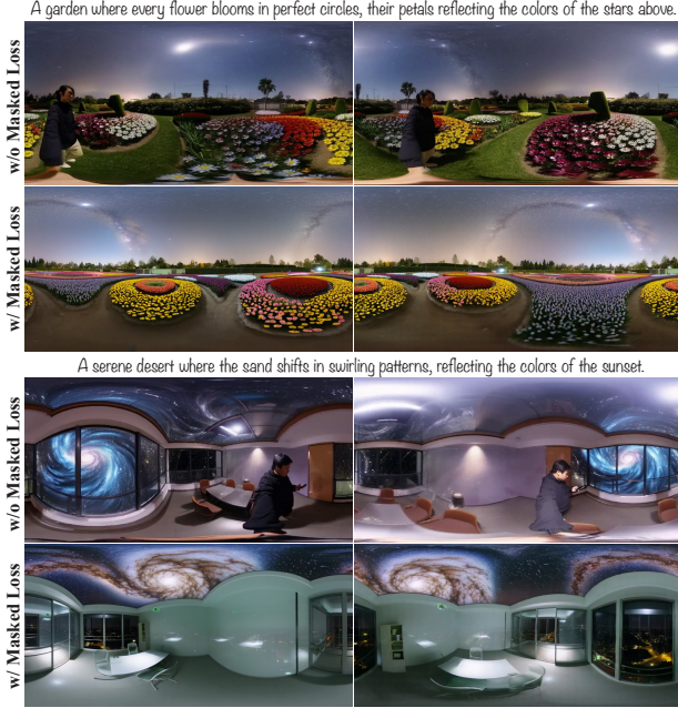
Fig. 4. We conduct an ablation study to evaluate the impact of the masked diffusion loss. This loss function effectively guides the model to generate only the pixels of the scene, eliminating the moving photographer present in the original video training data. As a result, it enables the generation of a complete 360° scene capture for reconstruction.
